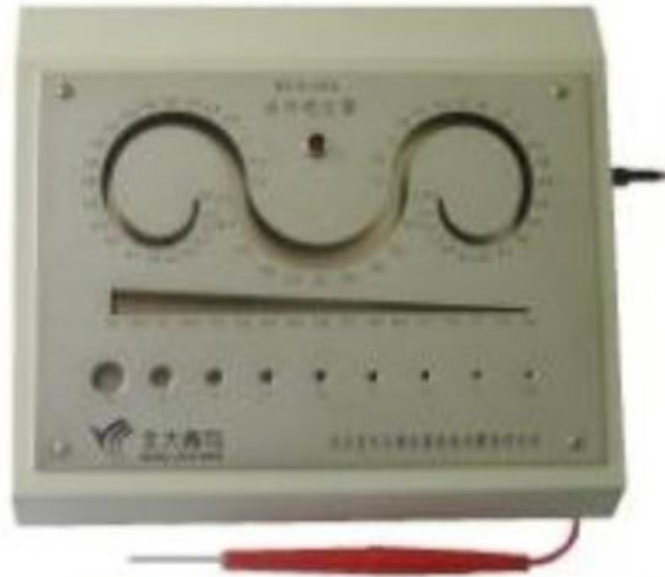
Figure 2. Apparatus for hand motion steadiness measurement
